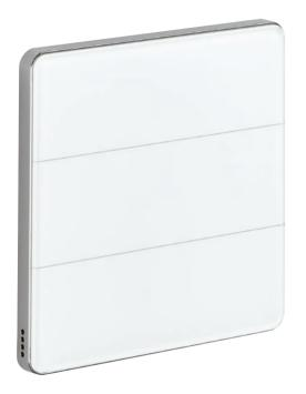
The AntumbraTouch range has a smooth glass finish and uses capacitive touch technology to detect finger pressure with no moving parts. Descriptive text and icon labeling describes functionality and is available in a range of languages.
