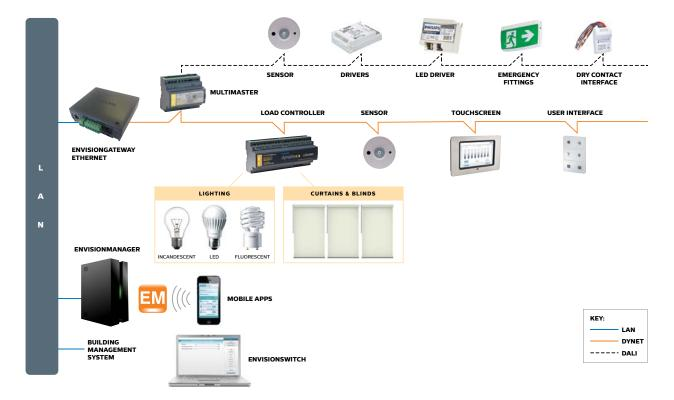
The system's distributed architecture offers excellent reliability and usability and provides flexible control of lighting and other building automation systems.
