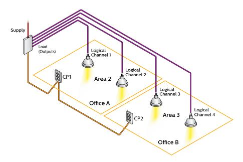
Grouping multiple individual control channels into different areas is essential in installations involving a large number of areas and channels. This saves time and work compared to systems in which every device must be addressed and configured separately.
