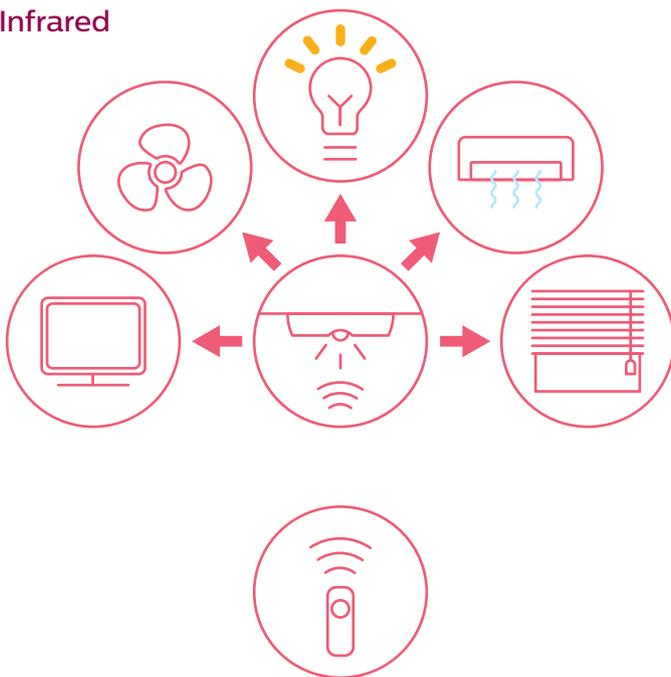
“ A Dynalite sensor enables IR commands to trigger complex pre-programmed tasks across the entire network ”
