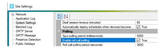
When System Manager is configured to detect offline devices, this information needs to be forwarded to the BACnet gateway. In the SM configuration tool, **Site settings > System Settings > Polling > Send DALI driver and Lamp failure aggregated for the whole site** must be set to True.
