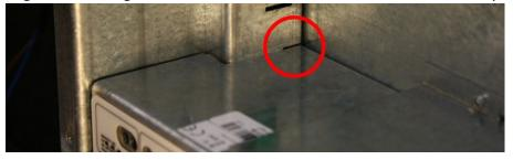
4. Secure the module using the fixing screw on the right. The unit should sit securely with no movement.
