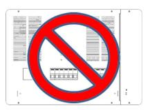
The DMC2 requires an air gap of at least 200mm (8 inches) on all sides of the front cover for adequate ventilation. This gap also ensures that the device is serviceable while still mounted.
