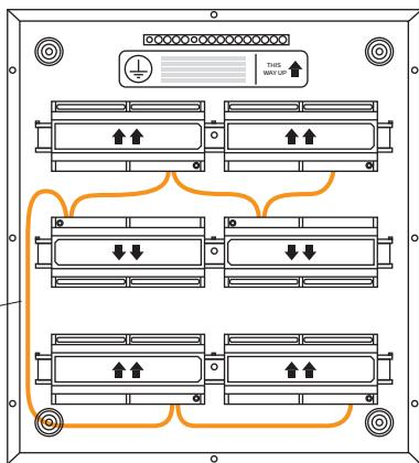
Refer to product label for Earth bar, wire gauge and torque ratings.
